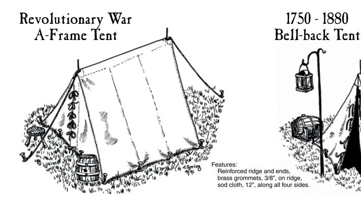
A bell-back tent is an A-frame tent with no back door. Instead, the back wall is made of three triangular panels staked out to increase floor space 24 to 36", without using larger poles. A-frame tents were used during the Revolutionary War, in fur trade rendezvous camps, during Earlier in appearance than other A-frame tents, it can be used in Revolutionary War encampments, fur trade rendezvous, Civil War reenactments, and at 1870 Indian War campaign camps.
