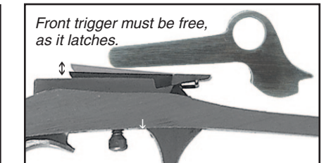
File the tip of the mainspring, if necessary, to increase rear trigger back lash (free play). Or adjust the back lash screw, if fitted.
