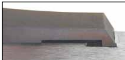
Easily form a raised dovetail for a rear sight.
